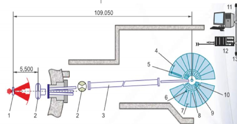
Ni, mirror, vacuum Neutron guide 50x160 mm<sup>2</sup> Guide aperture 4.6x10<sup>6</sup> n/cm<sup>2</sup>/s Thermal neutron flux at sample position 0.4 - 7.0 Å Wavelength range 10°-170° Scattering angles range ω=0-130 meV Energy transfer range (INS) 109.5 m Moderator - sample distance 0.815 m (INS with Be-filter) Sample - detector distance 1.015 m (INS with single crystal) 1.415 m (neutron diffraction) Resolution  $\Delta \omega / \omega = 2-4\%$ Inelastic scattering
